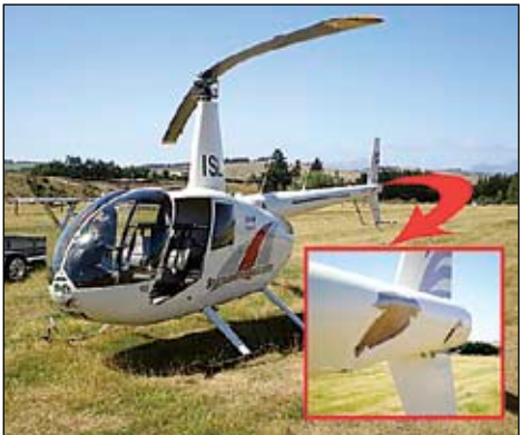
The R44 Raven II's tail rotor was destroyed, but the empennage remained intact.
